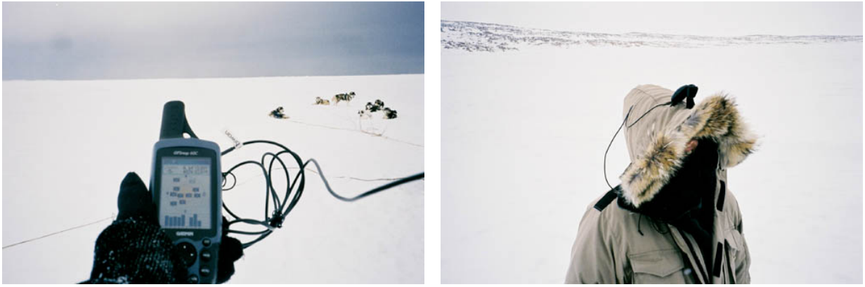
Figure 3-7: Garmin GPSMap 60C was used to track the sea ice routes traveled throughout all research trips (left). In order to maintain effective AA battery life the GPS was kept inside my parka for warmth, and an external antenna was attached to the top of my hood (right) to ensure clear reception. (photos: Gita Laidler (left) and Kristiina Alariaq (right))
