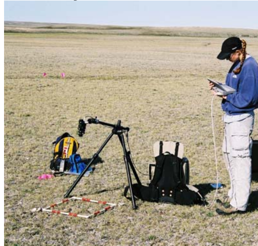
Figure 3.9 – Acquiring surface spectral measurements with the portable spectro-radiometer
